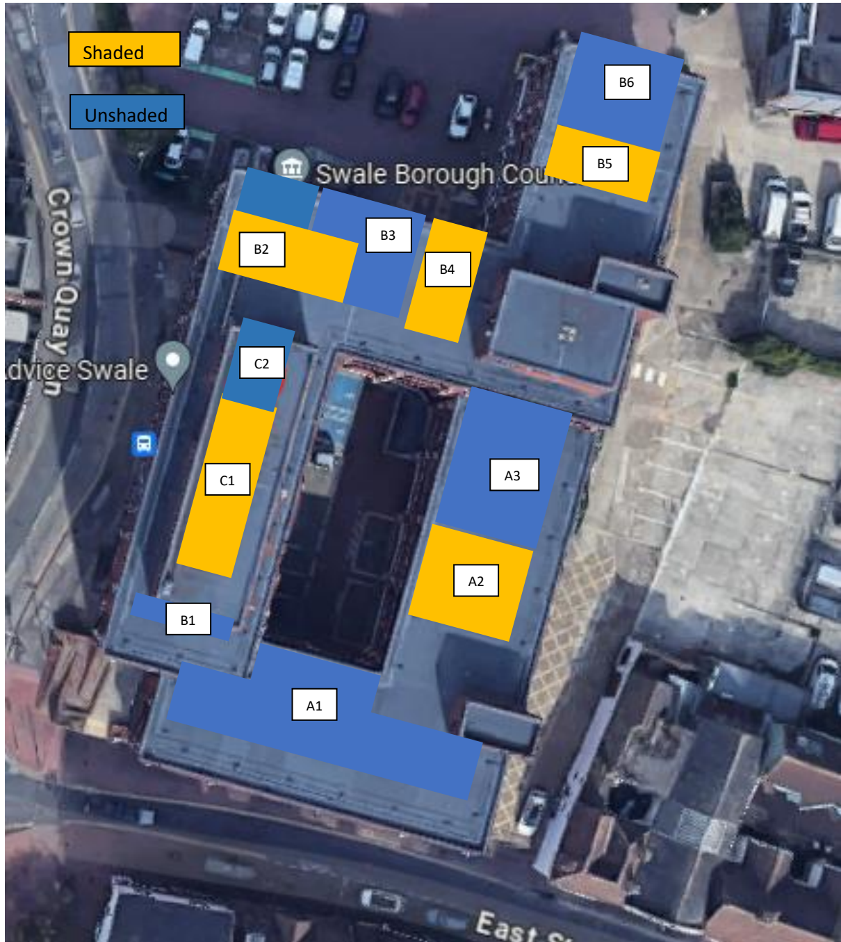
Figure 1 – Swale House Roof PV Layout
